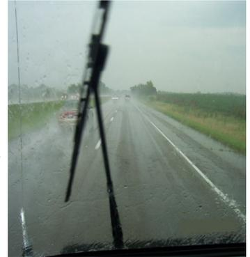
While daily pre-trip inspections of trucks are to be performed, particular attention should be given to the condition of wiperblades. After a long winter of salt and other road residue on the windows, wiper effectiveness can be greatly reduced. Make certain that they are in good condition before driving.
