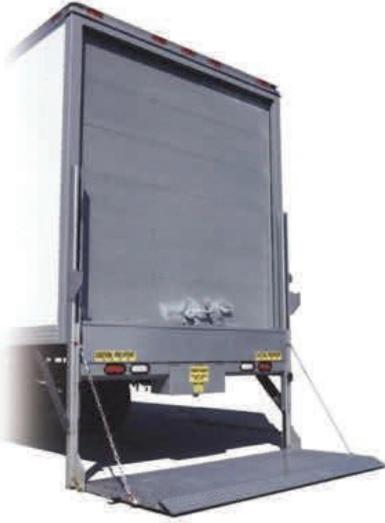
Some truck drivers use lift gates to assist in the loading and unloading of their trucks. Truck drivers who operate these lift gates need to be aware of potential pinch points since many of the operating mechanisms have exposed moving parts.
