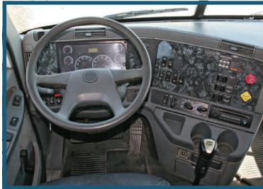
good idea to document every inspection. Review the previous day's Driver Vehicle Inspection Report (DVIR) to ensure any defects that were noted during the previous trip were fixed or deemed not to be required for the safe operation of the vehicle.
