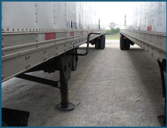
Even if the landing gear is maintained and undamaged, injuries can still occur, especially if the landing gear requires manual cranking. The most common injuries occur to the shoulders, back and wrists. Proper posture and technique can help reduce the potential for injury.
